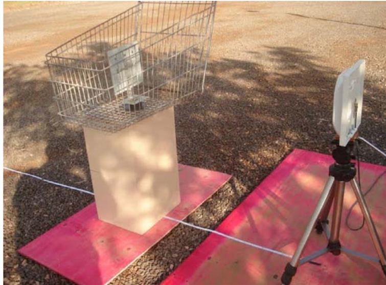
**Note:** Inside the metal box there is a base with a tag to verify the tags reading possibility in this kind of situation – on the right of the photo there is a RFID reader antenna
