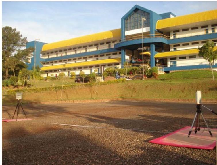
**Note:** On the left, a base with a tag and on the right a base with an RFID reader antenna
